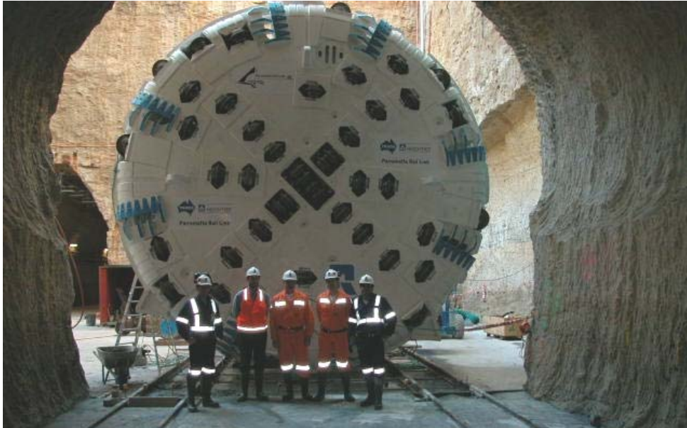
Figure 6-10 Rock Tunnel Boring Machine Face with Disc Cutters for Hard Rock, Australia.
