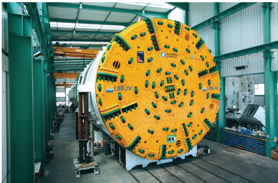
Figure D-9 above shows the cutterhead (about 40' diameter) of the Herrenknecht S-376 Double Shield TBM which is being used for the construction of Brisbane North-South Bypass Tunnel. See Table D-1 for more data about the machine (Herrenknecht).
