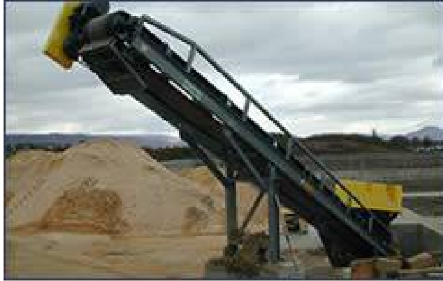
Figure 14-5 Surface Muck Storage Area
