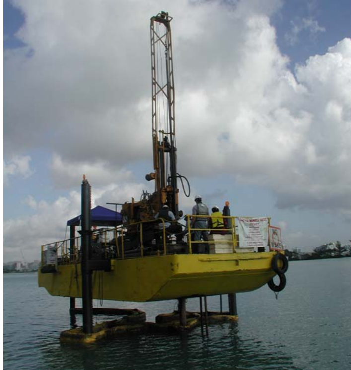
Figure 3-1 Water Boring Investigation from a Barge for the Port of Miami Tunnel, Miami, FL
