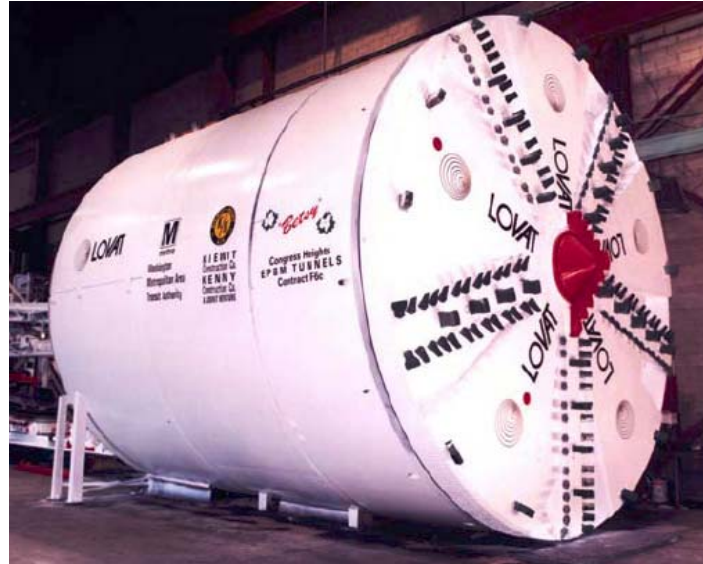
Figure 7-4 Earth Pressure Balance Tunnel Boring Machine (EPB) (Lovat).
