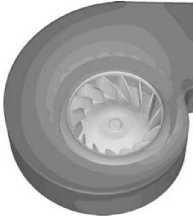
Fig. 5.12 Static pressure contours for flow through a centrifugal fan. (image courtesy of ANSYS, Inc. © 2008.)
