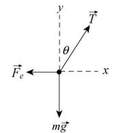
Examination of the geometry of the figure shown leads to  $\tan \theta = \frac{x/2}{\sqrt{L^2 - (x/2)^2}}$ .
