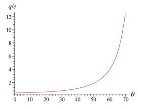
The graph suggests that q/e < 5 for  $\theta < 60^\circ$ , roughly. We can be more precise by solving the above equation. The requirement that  $q \le 5e$  leads to
